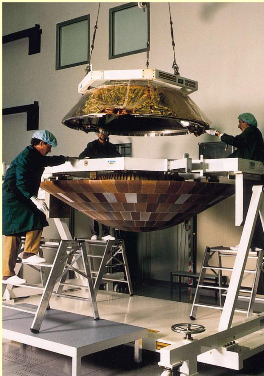
Protective shell. Heat-resistant tiles cover Huygens' curved front shield, to withstand the breaking and heating when it first enters Titan's atmosphere. The probe then discards the shield and the foil-wrapped back cover, revealing the instrumented section here seen nested in the shield.
